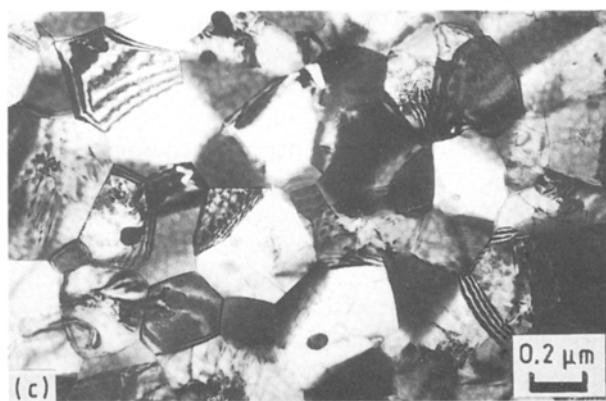
Figure 4 The fine structure of VT8 alloy strained at t = 700^\circ\text{C} and \dot{\epsilon} = 5 \times 10^{-4} \text{s}^{-1} . (a) \epsilon = 15\% , (b) \epsilon = 50\% , (c) \epsilon = 75\% .
